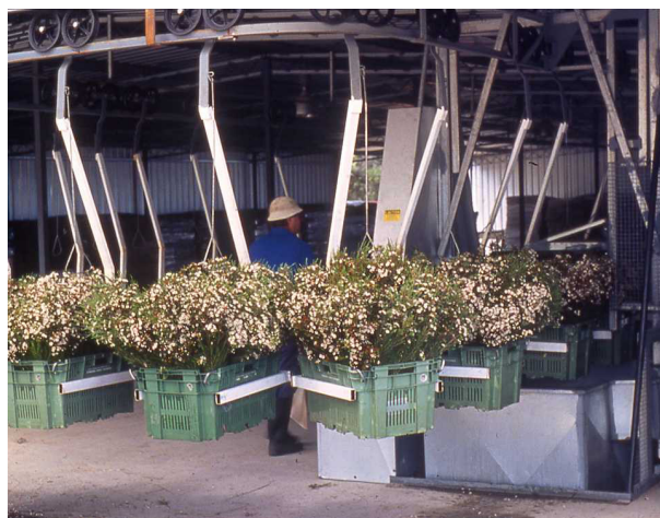
Figure 14.1. Dipping tank and draining board for treating a crate of 25 bunches of 60 cm long flower stems
