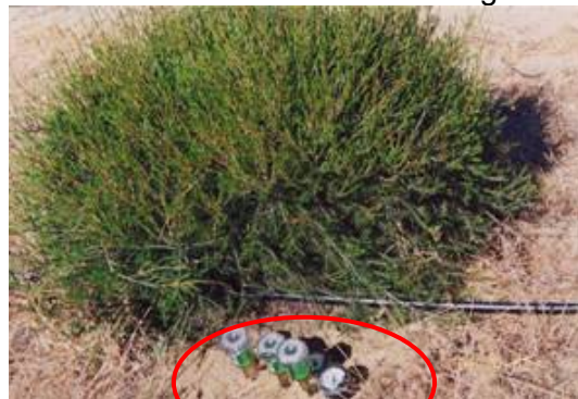
Figure 6.3. Tensiometers monitor soil moisture under a Pearlflower bush at 15, 30 and 60 cm
